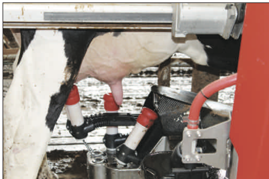
Another milking of an Ainsworth Holstein starts in their robot "parlor." The cows learn they can be milked when they choose. Guided by lasers, the robot washes the teats and attaches the milker. The family invested in the robots about a year ago in an effort to stay current in the dairy business.
