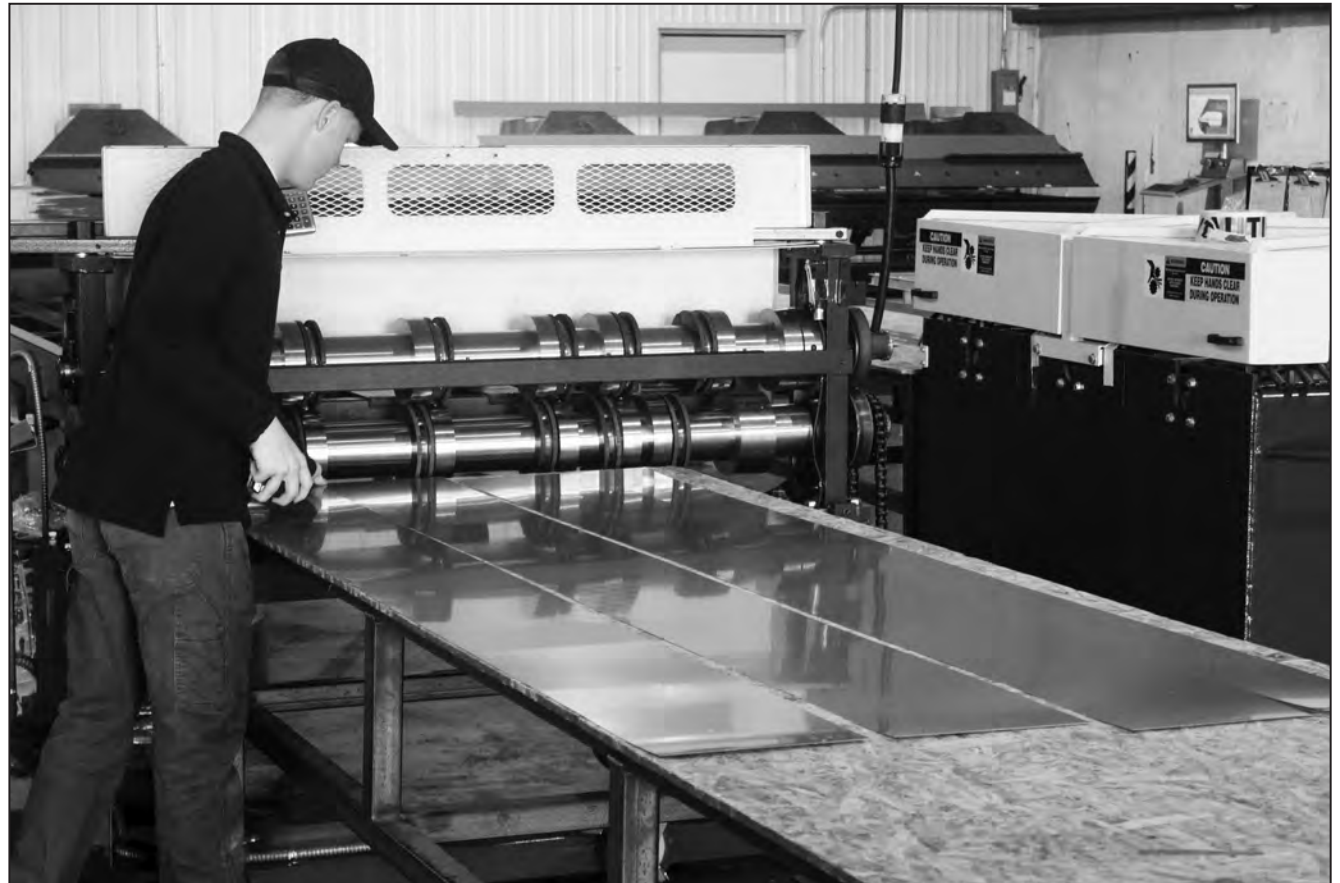
Richard Steinle, an employee with Hochstetler Metals, measures the metal roofing segments needed for a project during the Sept. 23 open house in Bonduel. Steinle trimmed a 41-inch segment into four pieces with 4-inch corners.
