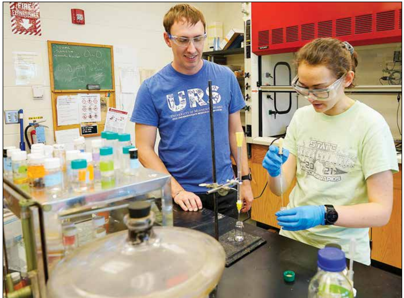
Angela Mosconi, right, performs a gravity filtration to separate solid impurities from a reaction mixture at Ripon College as Bryan Nell, assistant professor of chemistry, watches.
